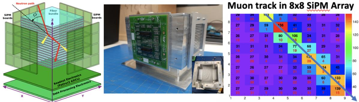
Fig. 1. (Left) SONTRAC Concept with two neutron scatters (red) and track imaging (yellow) with orthogonally stacked plastic scintillators readout by arrays of SiPMs. (Middle) SONTRAC prototype, (Right) Muon track through center of SONTRAC fiber bundle.
