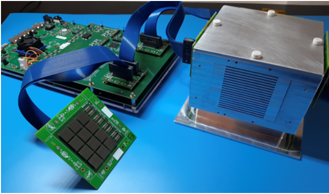
Fig. 2. New SONTRAC instrument prototype scintillator and 1mm SiPM detectors with 1.36mm pitch. SiPM board contains 32x32 1mm SiPMs with 1.36mm pitch and formed by a 16 KETEK carrier boards. The gap between the carriers is where the extra fibers (not being read) are located in the fiber bundle. The SiPMs are read out in strip (1D projections) to reduce the number of channels and encode the data.
