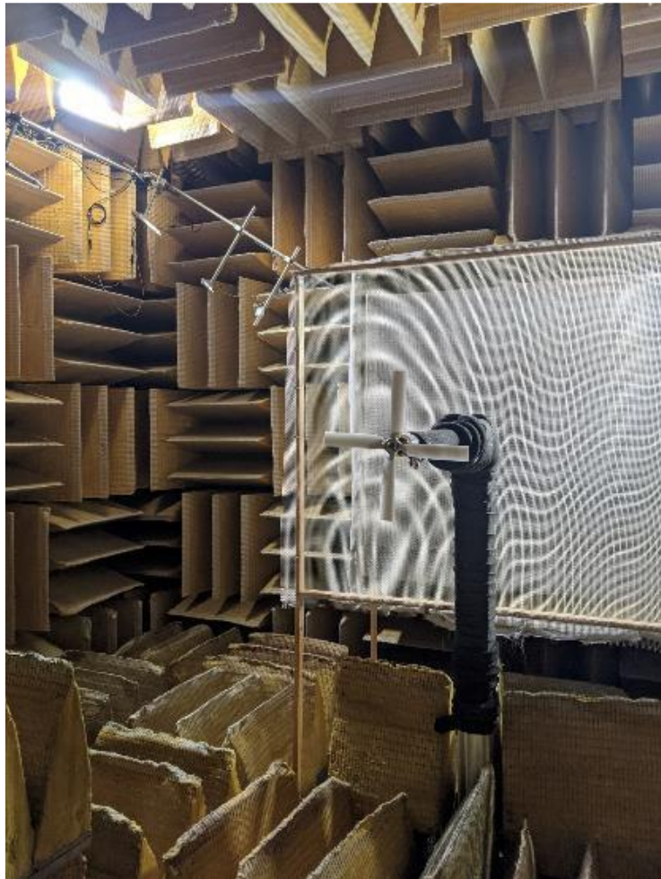
Rotor in Small Hover Anechoic Chamber (SHAC) at NASA Langley Research Center
