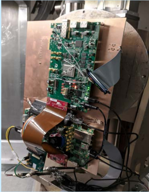
Fig. 4. Motherboard (KCU105) and daughterboard (PolarFire®) connection at the Lawrence Berkeley National Laboratory (LBNL) SEE vacuum chamber.
