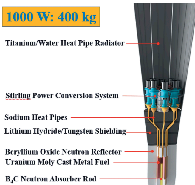
Fig. 1. Layout for 1-kW(electric) Kilopower system.
