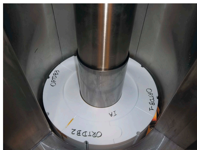
Fig. 6. KRUSTY BeO puzzle pieces, centering ring, and vacuum can, surrounded by radial shield.
