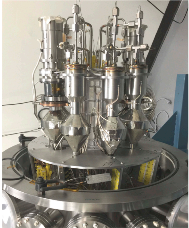
Fig. 2. The KRUSTY PCS consists of two 80-W-rated Stirling converters and six simulators (which mock the thermal behavior of the converters). At the bottom is the flange for the vacuum vessel. Over 100 TC wires and connections are packed between the flange and the PCS.
