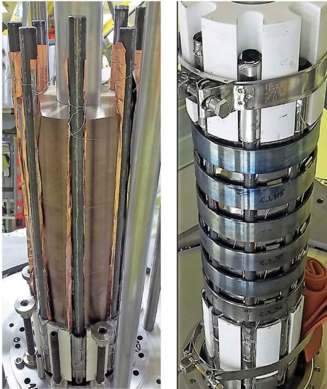
Fig. 8. KRUSTY core assembly: (a) heat pipes fitted within the slots in the HEU UMo fuel and (b) core after the installation of the Haynes 230 rings that clamp the heat pipes to the fuel (via interference fit). White BeO axial reflectors are seen on top and bottom. Some parts in the photographs are part of the temporary assembly fixture, which is later removed.
