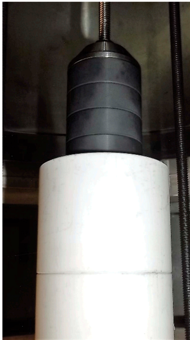
Fig. 5. B 4 C (dark gray) pucks stacked on top of BeO (white) axial reflector pieces.
