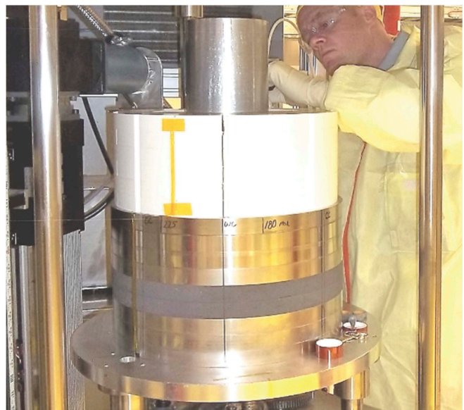
Fig. 4. The lower shielding and radial reflector being installed on the COMET platen, which consists of stacked 1-in.-thick rings of SS304 (shiny), B 4 C (dark grey), and BeO (white). Yellow tape holds TC wires.
