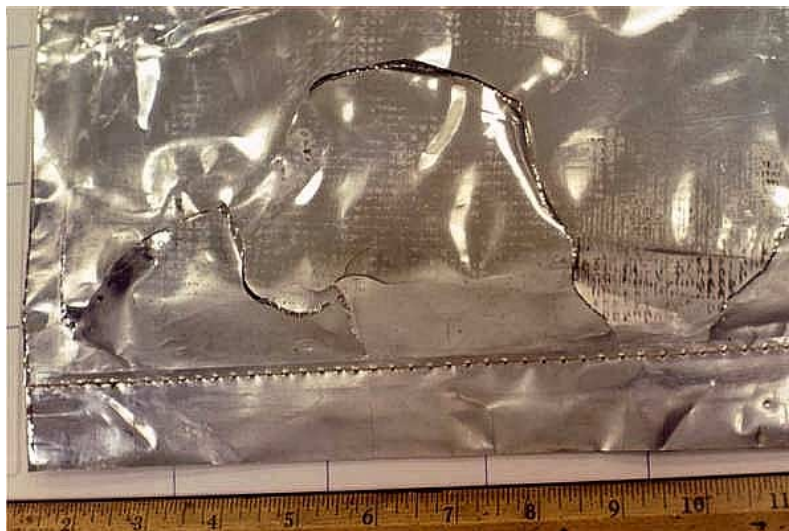
Figure 2. Cracks present in 5 mil thick Al-FEP Bay 10 MLI, photographed after retrieval during SM3A.
