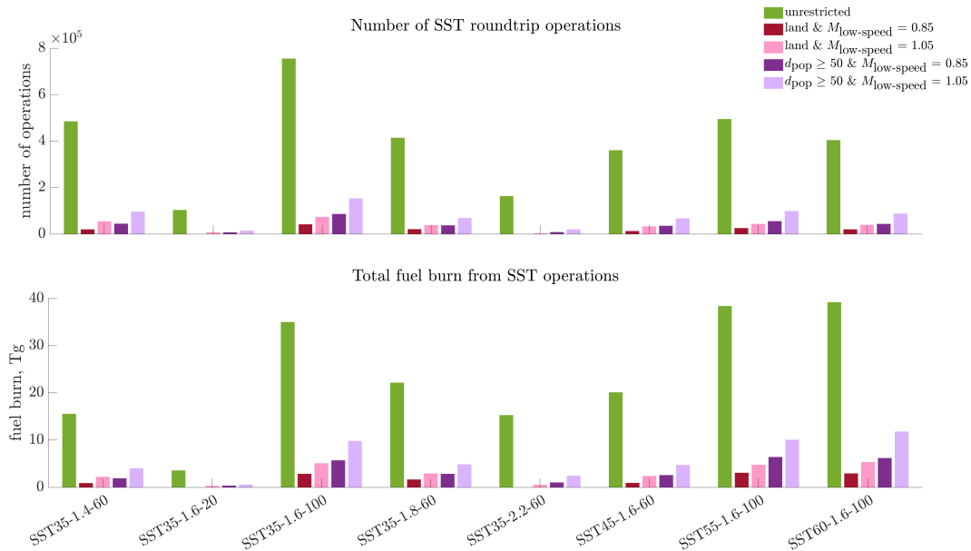
Figure 20: Global commercial supersonic market potentials and total fuel burn (only from SST) for the different notional aircraft, overflight restrictions and “low-speed” regimes.
