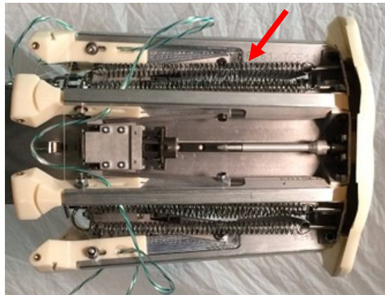
Figure 12. ADEPT Prototype showing Long-Travel Extension Springs
