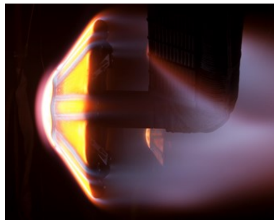
Figure 2. ADEPT ArcJet Heating Test
