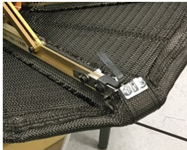
Figure 10: ADEPT Rib Tips with Kickoff Springs
