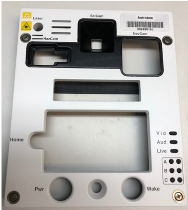
Free-Flyer Front Bezel (Made from Ultem 9085)
