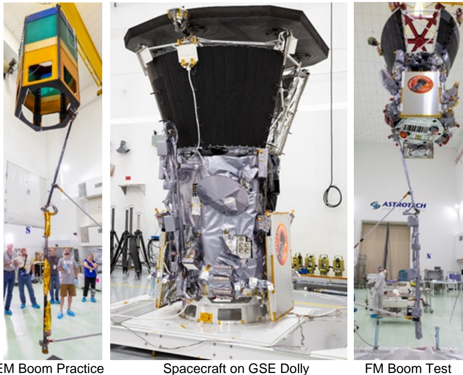
Figure 8. Boom Full Walkout Test on Spacecraft
