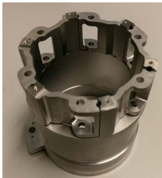
Figure 9: View of the chuck cam with integral flexures. The cam is machined as one piece using standard manufacturing processes including milling, drilling, turning, and band saw cutting. Despite the complex shape of the flexures, there was no need to utilize electrical discharge machining (EDM).
