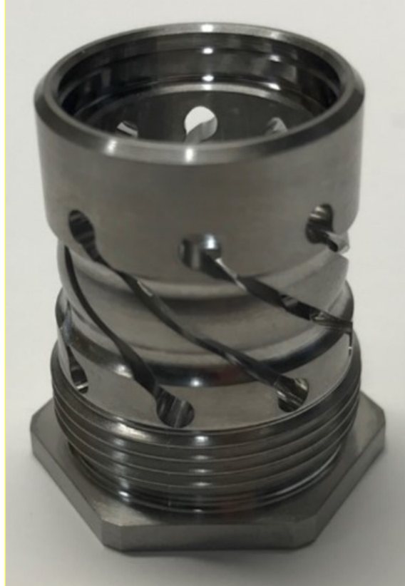
Figure 13. The absorber spring has a height of about 25 mm and a diameter of about 19 mm. The bottom end is threaded for installation into the output shaft that surrounds the selector. The top end includes a feature where a two-piece split collar and retaining ring are placed. Contact with the selector is made at this collar during impact. Regions of highest stresses are found at the round holes that terminate each slot.
