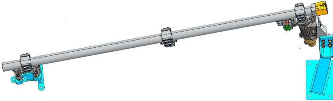
Figure 3: Top view: The clamshell mechanism that corresponds to the V1 FIELDS antenna position.
