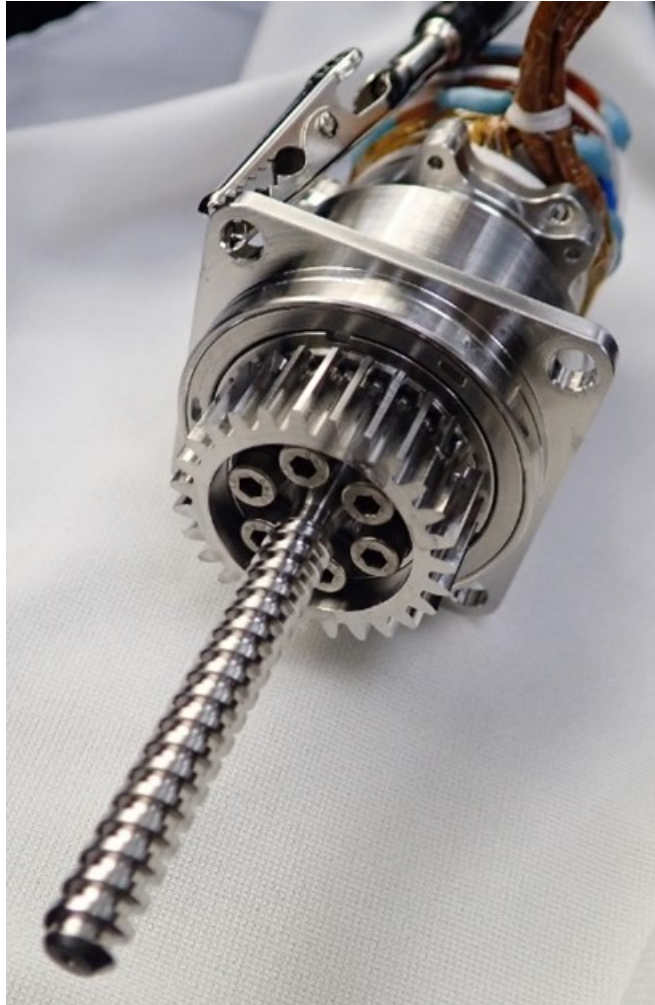
Figure 5. CBLO actuator and combined lead screw/spur gear output piece part. The lead screw drives a mechanism that interacts with the sample tube. The gear (via an idler) connects to STIG, allowing the selector to interface to the proper dual-output actuator interface.
