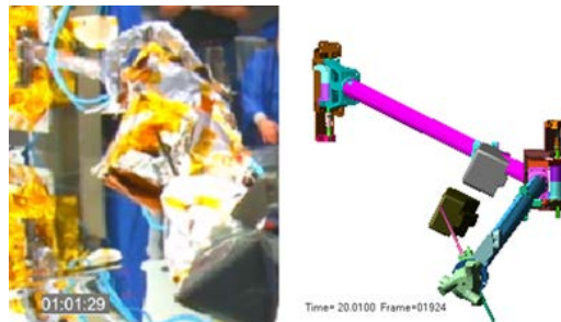
Figure 15. Mag boom Max Rebound Swing, Test at 21.0 sec and Analysis at 19.0 sec
