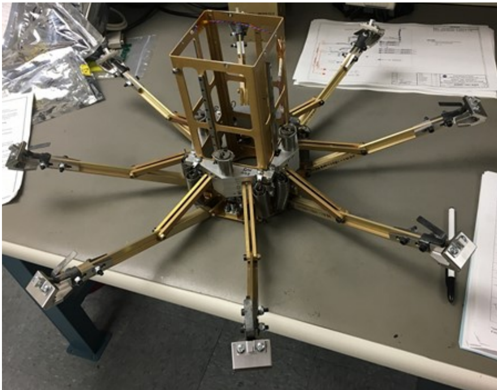
Figure 7. ADEPT SR-1 Ribs and Struts
