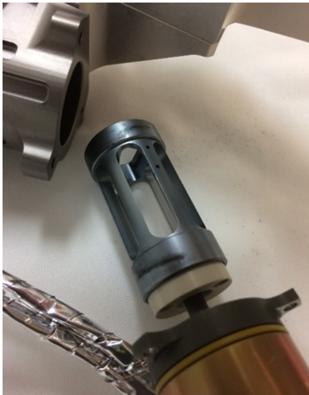
Figure 11: Removal of the sliding cup and pinpuller assembly, immediately after deployment anomaly
