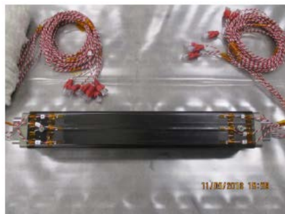
Figure 18 – Boom Tube Test Article
