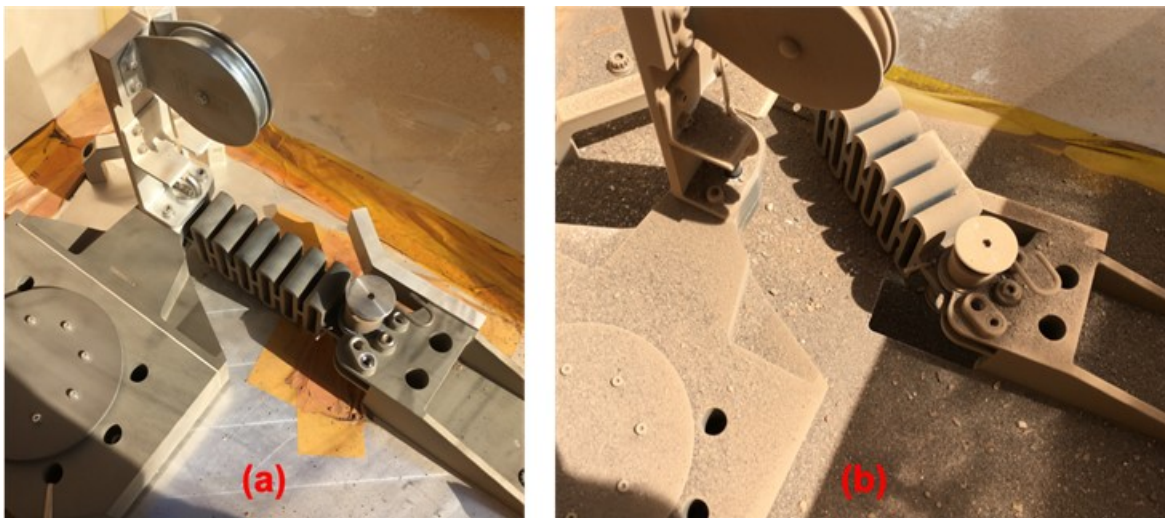
Figure 11. Showing the “dirty” test configuration: (a) showing the before the mechanism was coated with the Mars regolith simulate media, (b) after media circulation and deployment. This test was for the fault case with only the lower torsion spring having successfully deployed the flexure.
