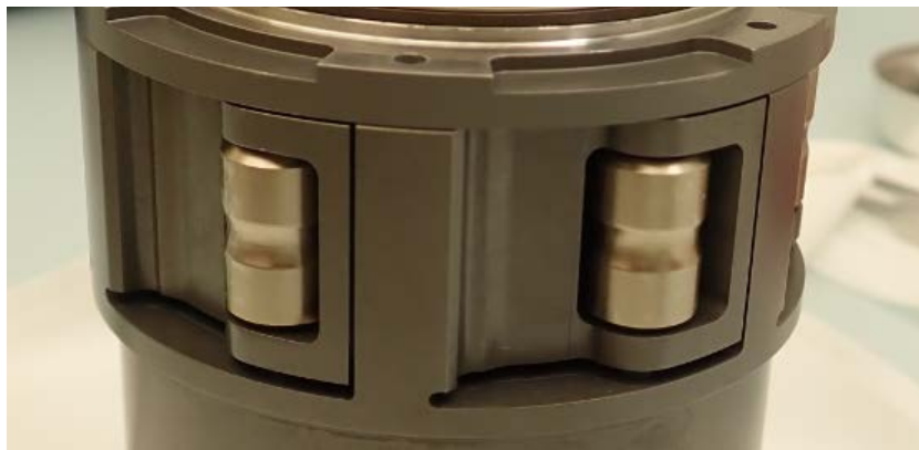
Figure 14: Detail view of cam rollers and concave central races. The rollers preload against the balls at these races. A concave race was added to each roller so as to minimize the Hertzian contact stresses generated under worst case loads such as would occur during rover slip or bit pullout.
