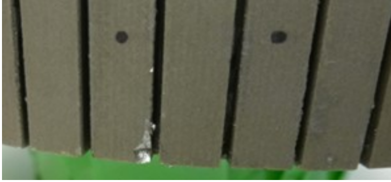
Figure 11. SmCo magnets damaged during AIT
