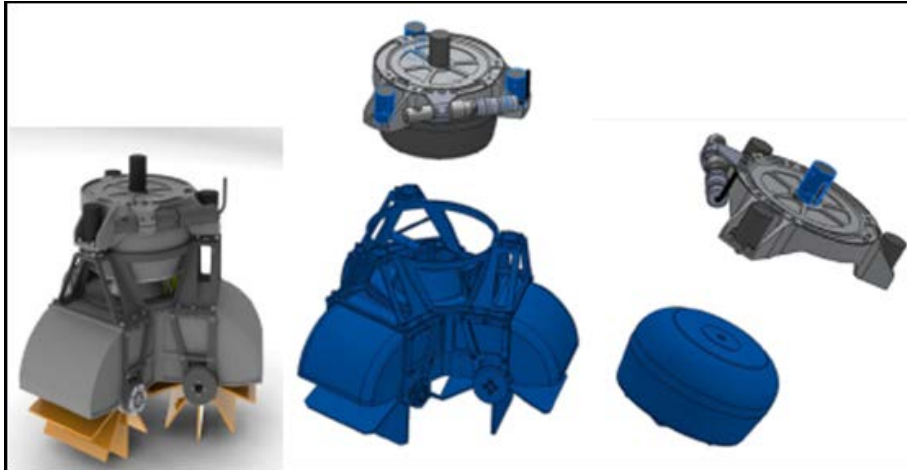
Figure 11. Sampling Tool Mechanism (left), 1st Disengagement (center) and 2nd Disengagement (right)
