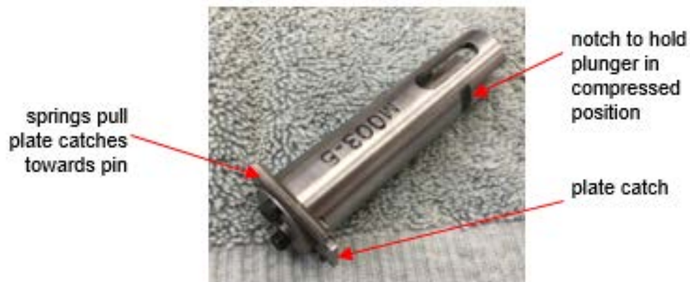
Figure 20. ADEPT Plunger Assembly with Notch for Latch
