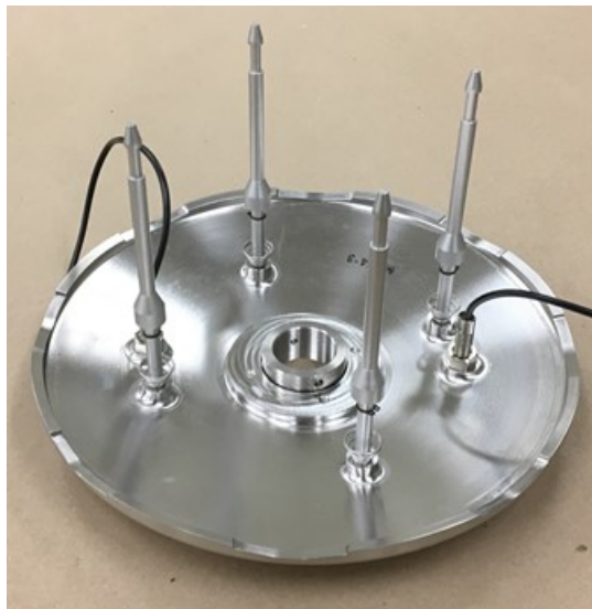
Figure 14. ADEPT Nose Cap with Pins and Proximity Switches
