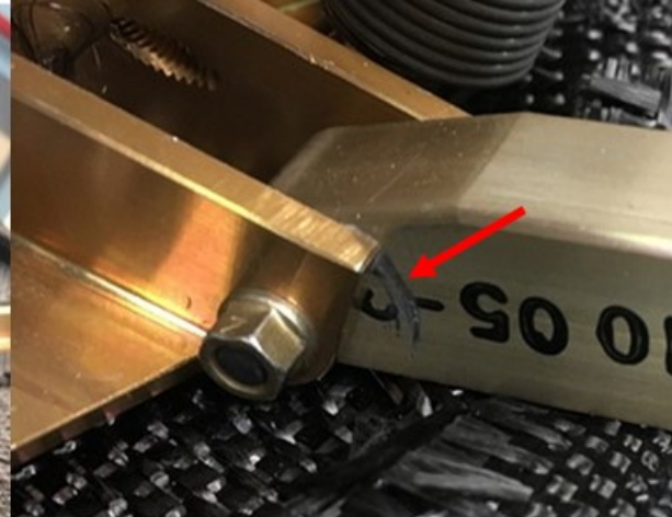
Figure 27: Wear at Pivot Joints
