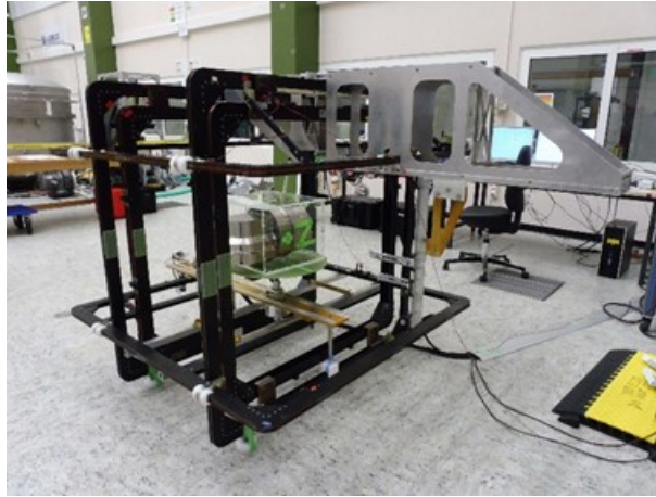
Figure 19. APM Protoflight model magnetic characterization test
