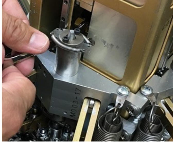
Figure 23: Fully Deployed ADEPT Showing Extended Plungers with Captured Pin Tips
