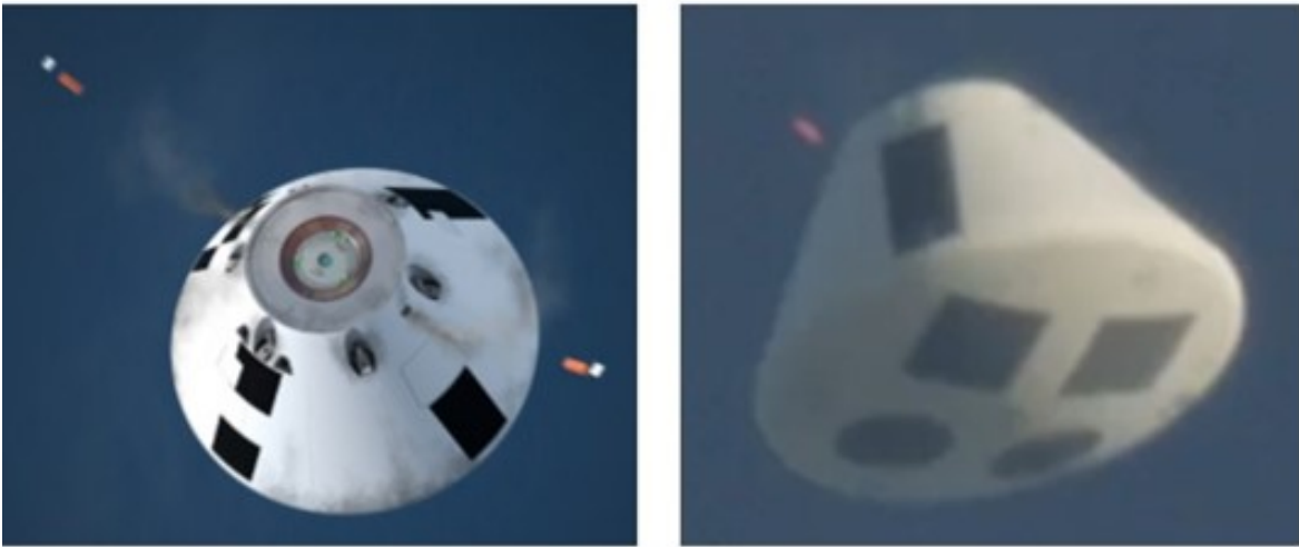
Figure 5. EDR ejections. Figure on the left is an artist rendering and the first on the right is an image from the actual flight.
