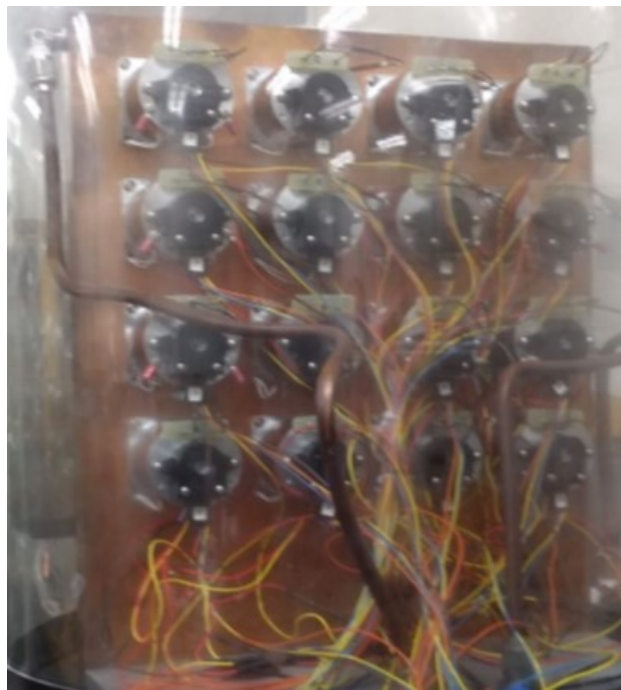
Figure 3. Test motors mounted on chiller plate and installed in bell jar.
