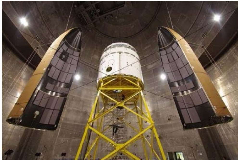
Figure 1: RUAG fairing test at NASA Glenn Research Center Plum Brook in Sandusky, OH [1]
