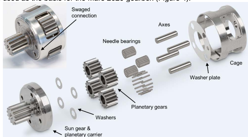
Figure 4. Exploded view of M20 planetary gearbox stage
