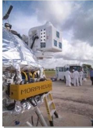
ALHAT Flash Lidar mounted on Morpheus
