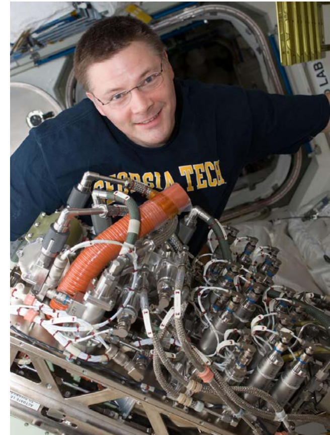
Astronaut Doug Wheelock installs the Sabatier CO 2 Reduction Assembly (CRA) on ISS. The CRA was returned to Earth in 2018. ESA's Advanced Closed Loop System (ACLS) launched in 2018, contains a Sabatier reactor.
