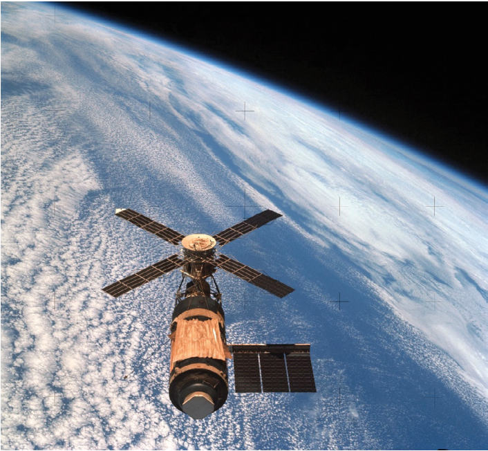
During launch of Skylab 1, there was a complete loss of the micrometeoroid shield from around the lab and damage to a solar array. Repairs made during the Skylab 2 mission included installing a sunshade for thermal control and releasing the damaged solar array.
