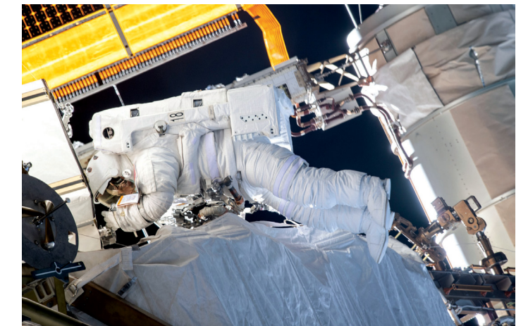
NASA astronaut Christina Koch installs Li-ion batteries in an ISS power system upgrade.
