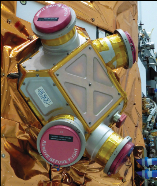
Busek cluster of four colloid microthrusters as flown on the LISA Pathfinder Mission. Source: ESA/Airbus
