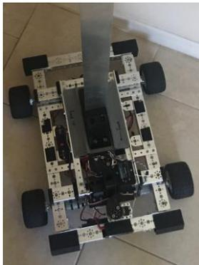
**Figure 3. Penny chassis.** The flat fixed pendulum is seen installed; both the original (black) pendulum holder and the new (grey) one are visible.
