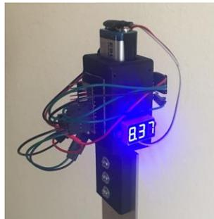
**Figure 4. Penny tip rate gyro assembly.** The voltage monitor, 9V battery, and Pro Micro are shown; the XBee and MPU6050 are on the other side of the assembly.
