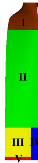
Fig. 6 Rotor blade split into separate FW-H surfaces (top view).
