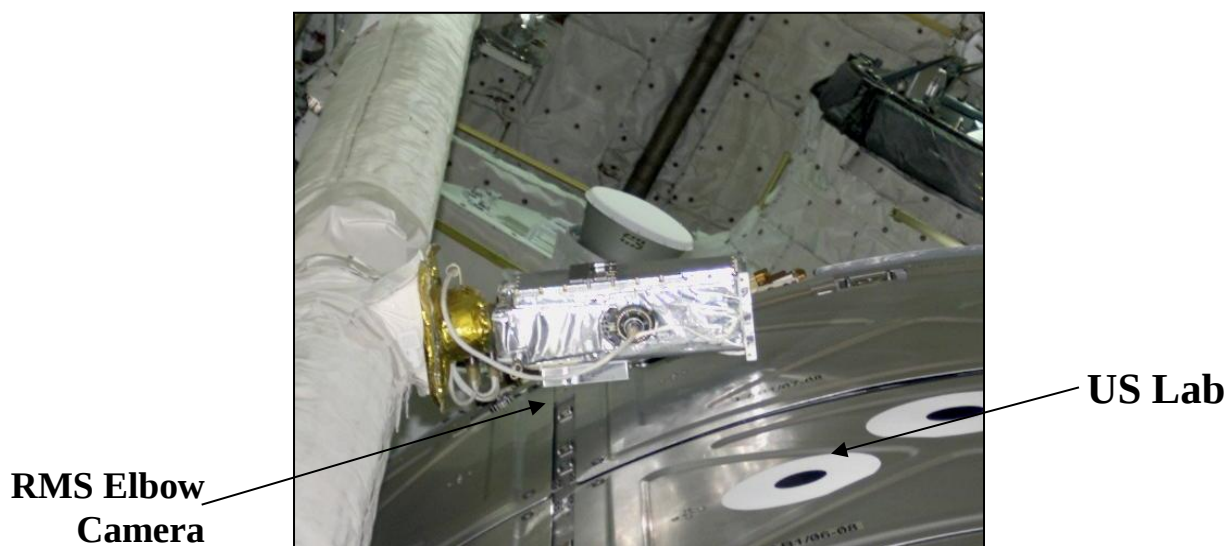
Fig. 2: Near interference between the RMS Elbow Camera and the US Lab Module
