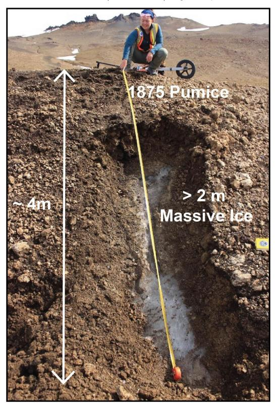
$\geq$  60 cm of ice has been found beneath the 1961 tephra deposit (pictured below) and deposited on top of 1875 materials.
