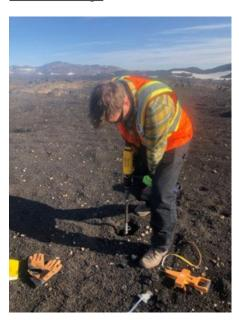
A hammer drill with an augur was used to retrieve core samples down to 1.5 m at locations where buried ice may have been detected by the GPR.
