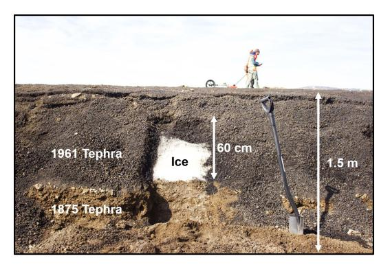
Traverses with the GPR at both 200 and 400 MHz antennas were taken at both of these locations.
