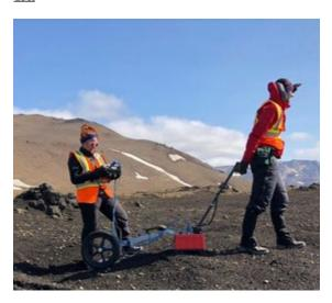
We conducted our surveys using the Geopysical Survey Systems Inc. (GSSI) ground penetrating radar antennas at 200 MHz and 400 MHz (400 MHz pictured above). These were attached to a survey wheel where data were collected as a time-series at 100/m along a traverse. A Trimble Geo7x handheld GPS was used to track the GPR position along the traverse.
