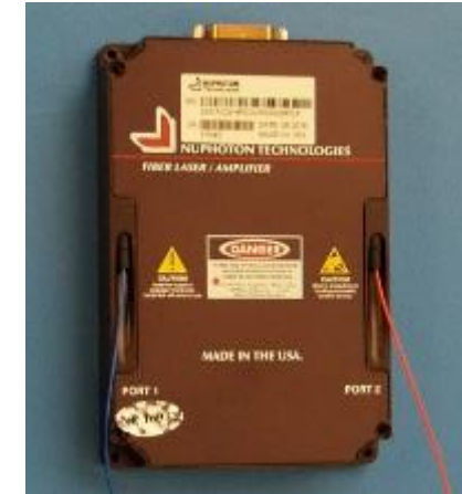
~1W Erbium Doped Fiber Amplifier Optical C-Band (~1550nm)
