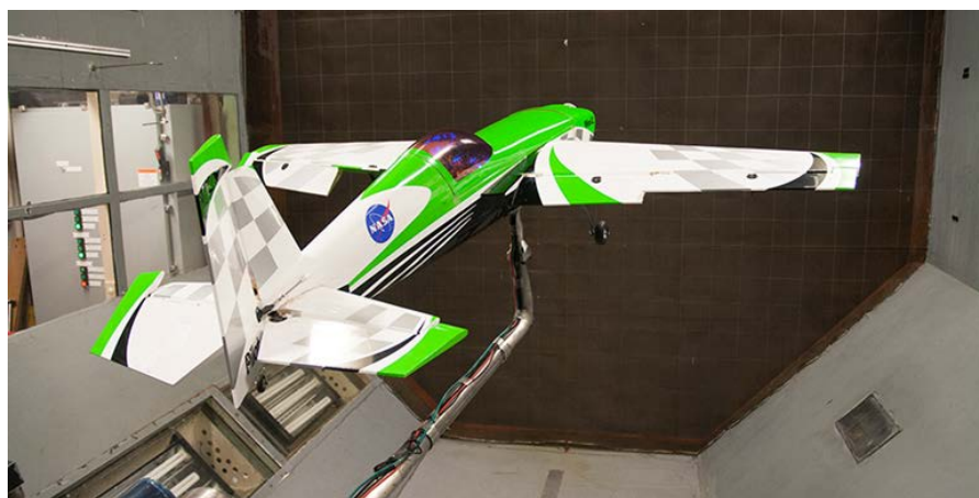
Figure 1. Conventional aircraft (Mini E-1) in the NASA Langley 12-Foot Low Speed Tunnel.
