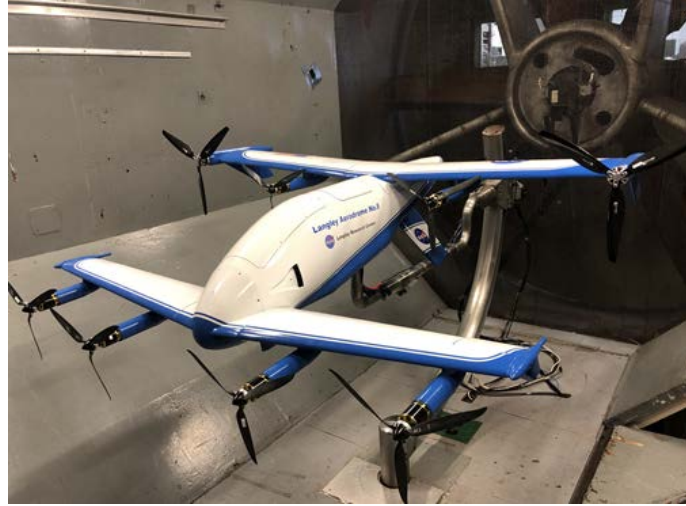
Figure 2. UAM aircraft configuration (LA-8) in the NASA Langley 12-Foot Low-Speed Tunnel.
