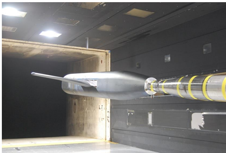
Figure 4: The NASA Juncture Flow test article installed in the NASA 14- by 22-Foot Subsonic Tunnel.
