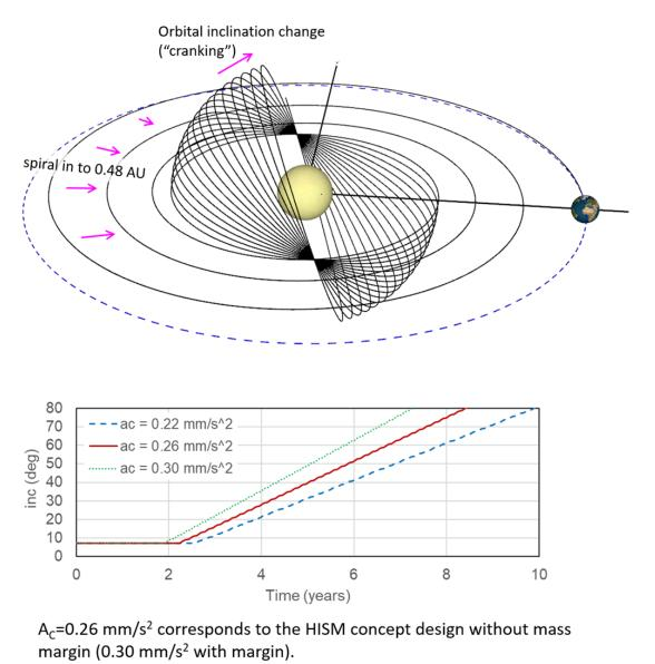
The mission design is based on the Solar Polar Imager study. The mission consists of a spiral-in phase to 0.48 AU ecliptic orbit, followed by a cranking phase to gradually increase the orbital inclination. **Full science observations start at the beginning of the cranking phase.**
