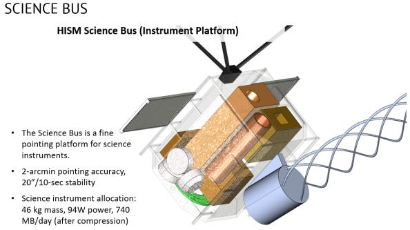
• Shown here are a magnetograph / helioseismology instrument, coronagraph, deployable boom with magnetometers and solar wind / ion instruments, and electrical antennas.
