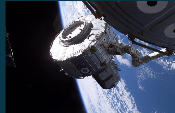
ISS Quest Joint Airlock installation on STS-107
