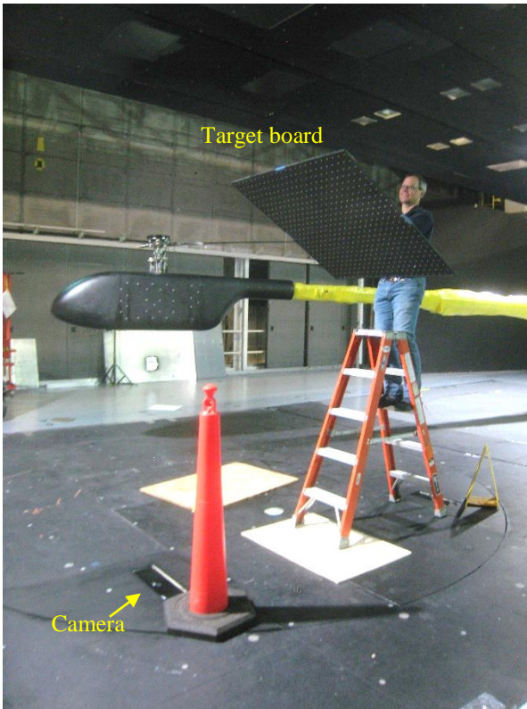
Fig. 5 Imaging target board for internal calibration of camera. Model has been yawed out of the way.
