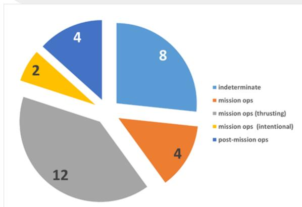
Mission operations can include thrusting or coasting prior to payload separation and avoidance or stage passivation activities. In two cases the event was intentional and are so noted. The other two categories are post-mission operations and indeterminate, in which the exact timing of the event is not possible.
