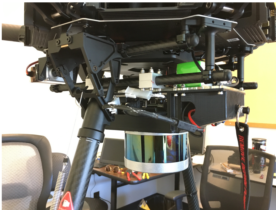
Figure 3: Fully enclosed Gen 2.1 payload mounted on the M600 Pro.
