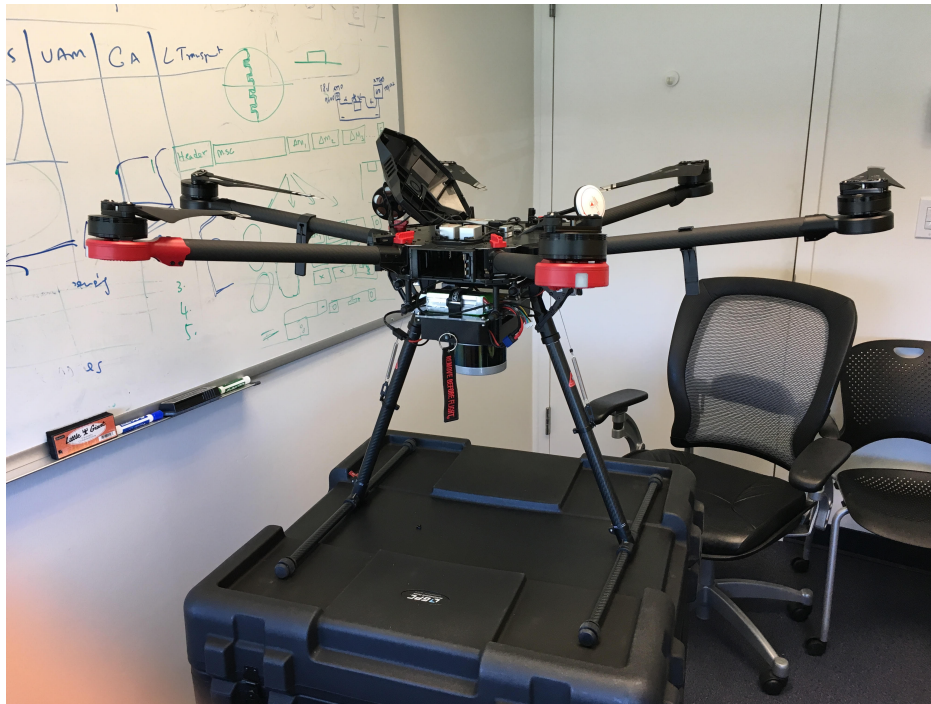
Figure 1: Gen 2.1 payload mounted on the M600 Pro.
