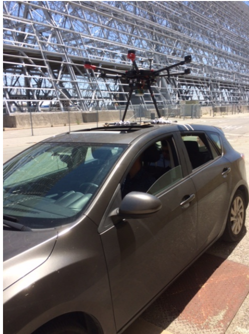
Figure 12: Drive test rig where the M600 Pro was secured to a car to test LIDAR point cloud collection with the Gen 2.1 payload.
