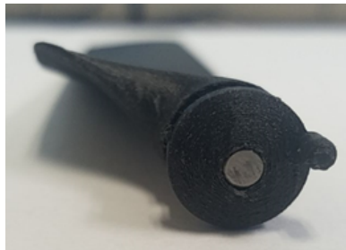
(b) Blade root design with aluminum spar
