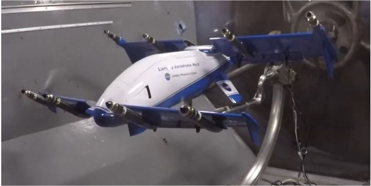
Fig. 1 Isometric view of the LA-8 in the NASA Langley 12-Foot Low-Speed Wind Tunnel.
