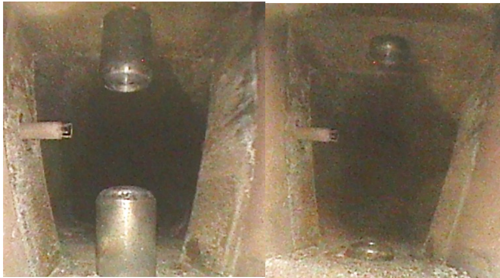
Figure 54. TDLAS and Dual-TC probe installed in rig (view is forward looking aft): (left) initial probe configuration tested with 1" separation, (right) final configuration with 2.5" separation
