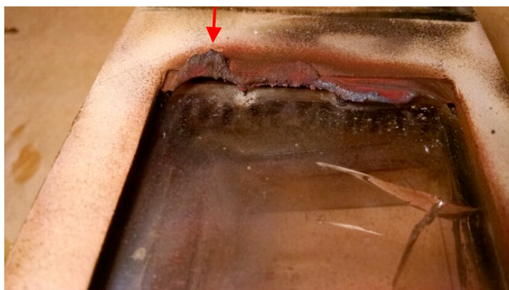
Damage to slot injection lip early on due to lack of cooling air flow while increasing rig pressure (repaired)
