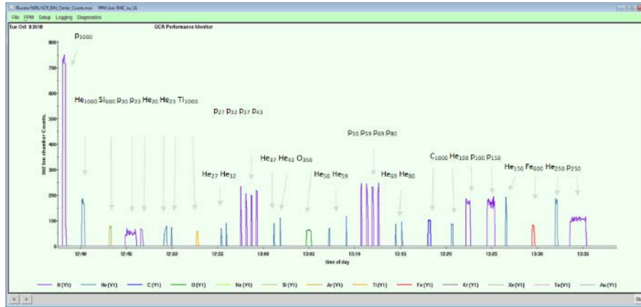
Fig 10. Computer screen shot measuring GCR simulator doses per ion for the 20.8 mGy cycle. On average, the cycle took ~70 to 75 minutes of which over 50 minutes were devoted to beam switching.
