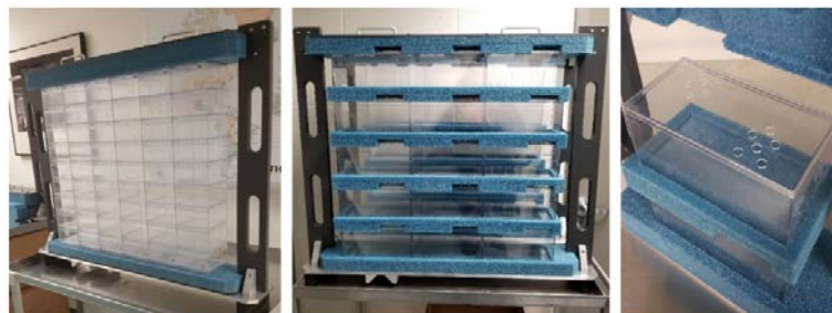
Fig 11. Housing array for mouse (panel A) and rat (panel B) irradiations in the 60 x 60 cm 2 beam. Exposure boxes, made of ~2mm thick polyethylene, stack together and are held in an array using a fabricated frame structure. (C)
