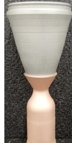
Multi-material combination with L-PBF and DED (RAMPT Project)
