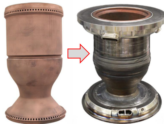
EB-DED Inco 625 Jacket on L-PBF GRCop-84 Liner
