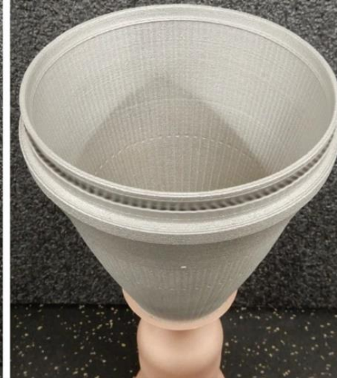
Multi-material combination with L-PBF and DED (RAMPT Project)
