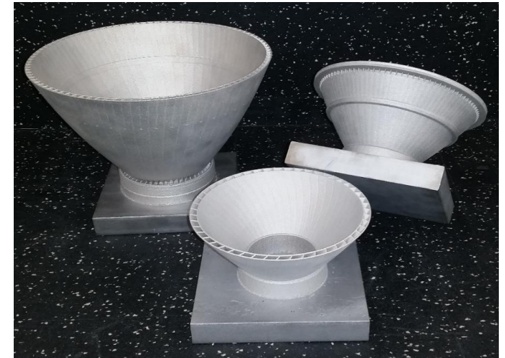
40" (1.016 m) and 38" (0.965 m) height nozzle with internal features built in 30 days using LP-DED
