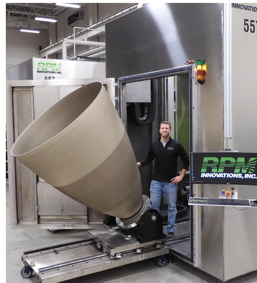
60" (1.52 m) diameter and 70" (1.78 m) height 90 day deposition
