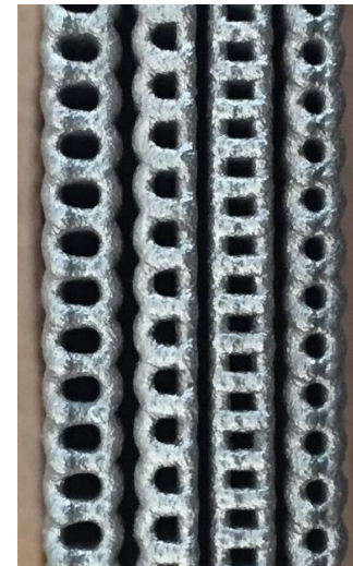
40" (1.016 m) and 38" (0.965 m) height nozzle with internal features built in 30 days using LP-DED
