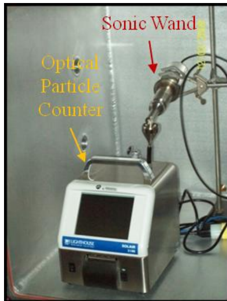
Optical particle counter and sonic wand (From Method and Apparatus for the Quantification of Particulate Adhesion Forces on Various Substrates by Christopher J. Wohl, Brad M. Atkins, and John W. Connell (October 2010))
