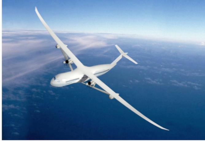
**Figure 1. Boeing SUGAR Truss-Braced Wing (TBW) Aircraft Concept**
