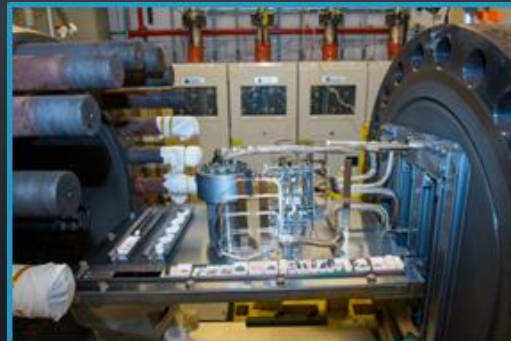
LLISSE lander set up for system test (4)
