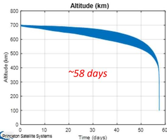
Deorbit time versus altitude and percentage of full boom deployment: uncontrolled and sun-pointing
