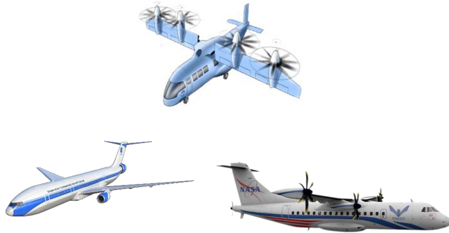
Figure 1. Considered aircraft concepts: tiltwing (top), STARC-ABL (bottom left), and PEGASUS (bottom right), not to scale.
