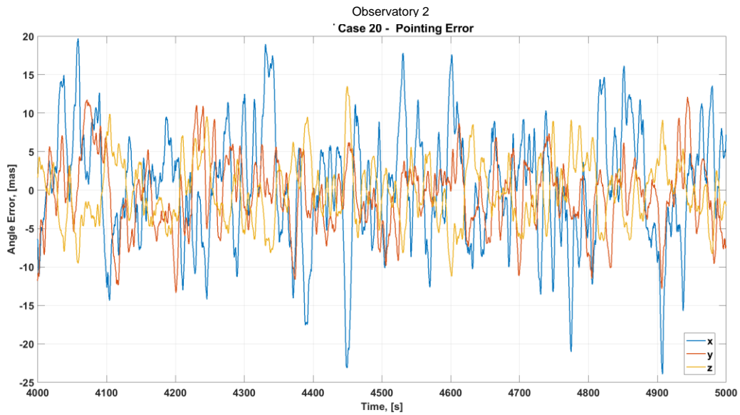
Figure A.1-19. Case 20 Steady-State Pointing Error in mas
