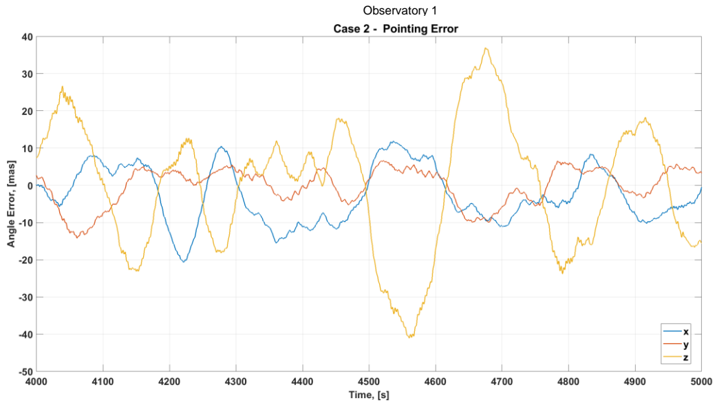
Figure A.3-3. Case 2 Steady-State Pointing Error in mas
