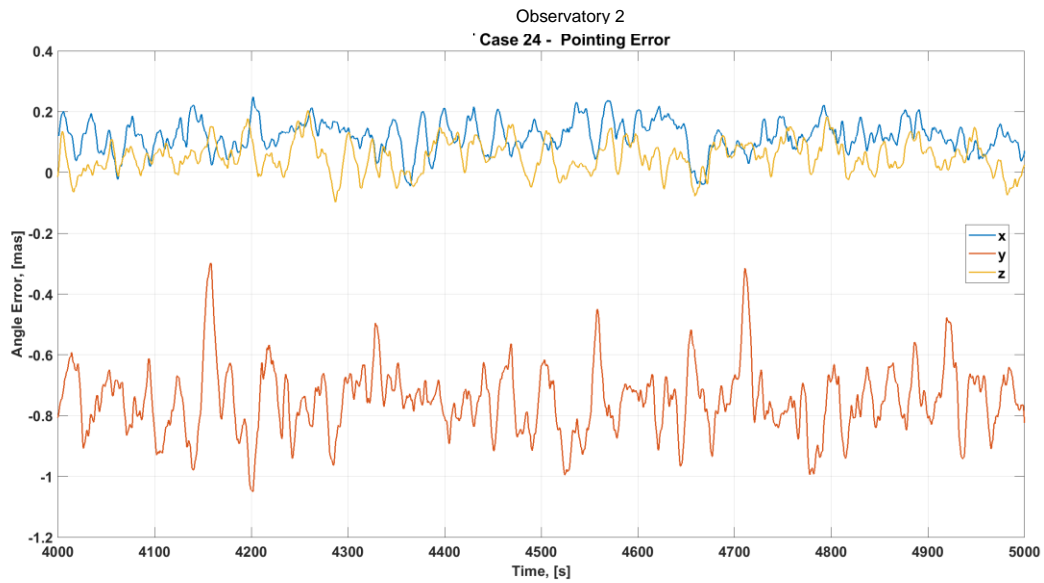
Figure A.1-23. Case 24 Steady-State Pointing Error in mas
