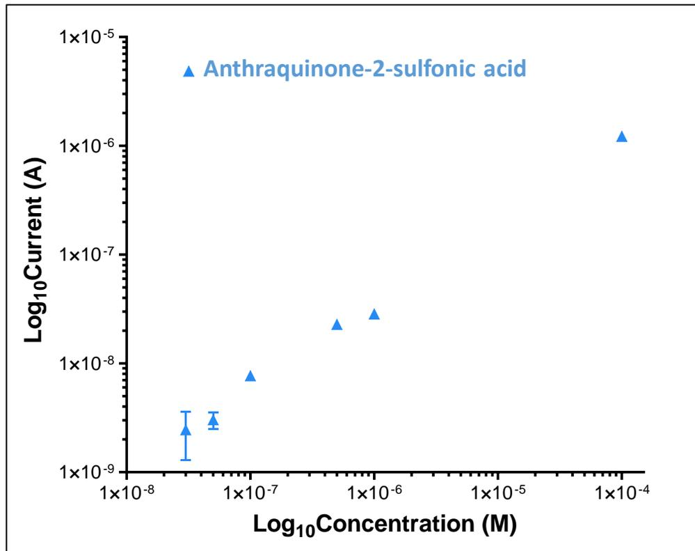
Limits of Detection Found Using Differential Pulse Voltammetry
