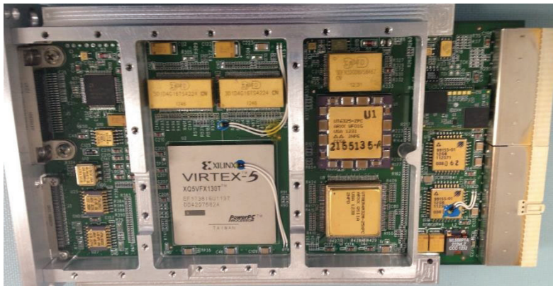
Figure A.3-4. SpaceCube v2.0 Processor Card
