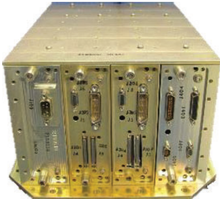
Figure A.3-5. SpaceCube v2.0 Computer
