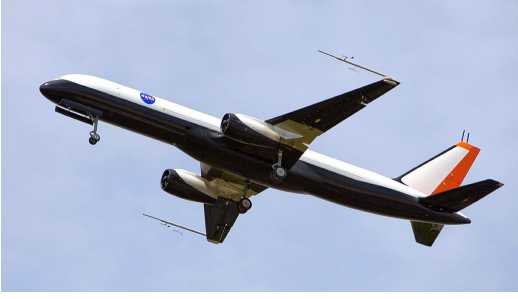
Figure 1. T-2 subscale jet transport aircraft (credit: NASA Langley Research Center)
