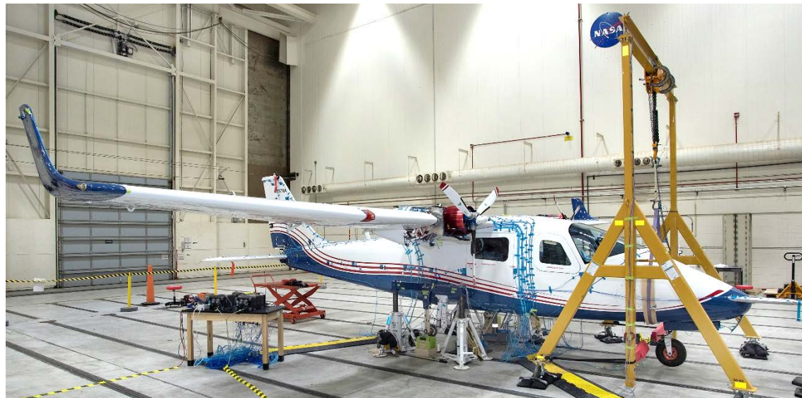
X-57 Mod II GVT, Conducted at NASA Armstrong Fall 2019
