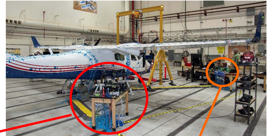
LAN-XI DAQ Fwd Aircraft Setup
