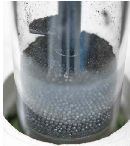
Catalyst beads, particulate carbon & attritor are visible at base of subscale reactor
