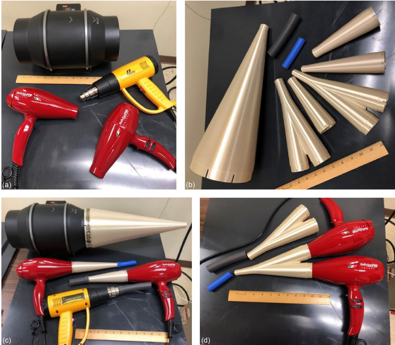
Figure 2.—Equipment used to produce forced air during charging experiments. (a) Fan used for cooling, Volare® ionic hair dryers (BaBylissPRO®), and Ponie temperature-programmable heat gun. (b) Adapters and high-temperature tubing used for directing airflows. (c) Adapters connected to forced-air equipment. (d) Dual-stream merging adapter connected to twin ionic hair dryers
