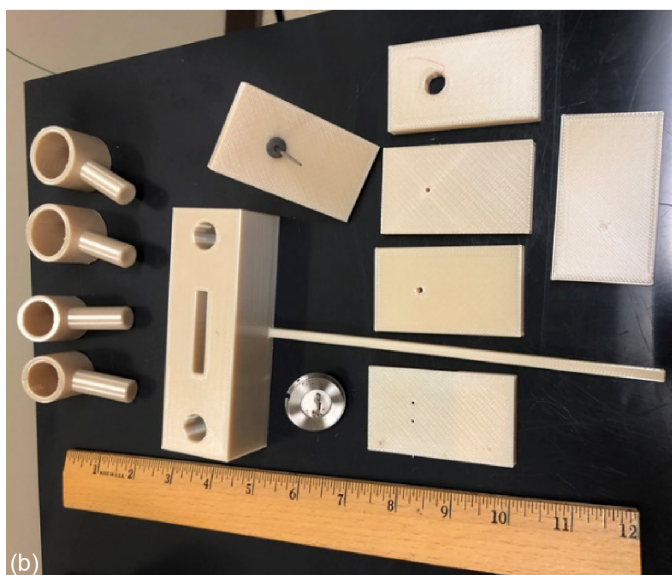
Figure 11.—Three-dimensional printed emitter-holder setup and components. (a) Setup corresponding to the Through Current (TC) configuration, loaded and clipped Gen 4 sample holder, loaded Gen 2 electrode holder connected to electrical ground, and LaB 6 -loaded emitter holder. (b) Emitter holder including built-in alignment track and associated accessories such as air-hose holders, LaB 6 emitter, and insert-card emitter adapters including one with loaded needle through nylon-foam cushion.
