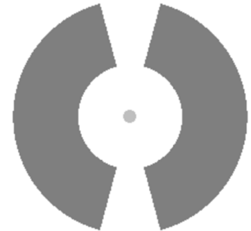
c) Focal plane mask design with bowtie through holes and a reflective central spot with a phase dimple for LOWFS
