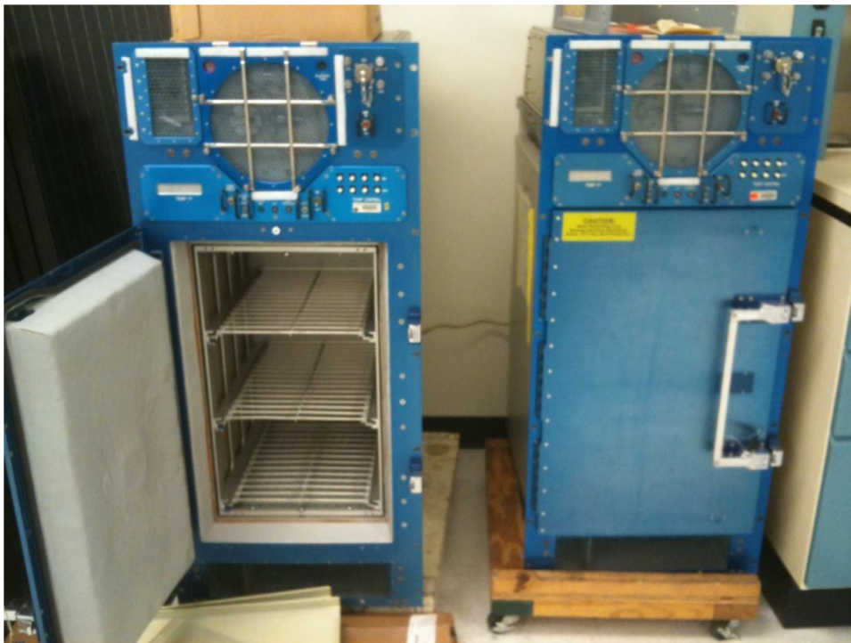
Fig. 3. LSLE refrigerators were flown in the 1990s on space shuttles.
