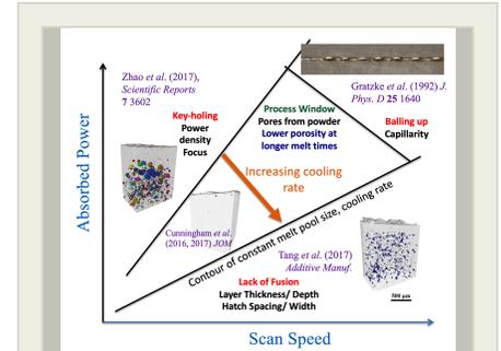
The figure shows an example of how the defect structure in laser powder bed fusion machines varies in a systematic but highly non-linear manner across power-speed space. In one corner, lack of overlap of melt pools induces lack-of-fusion...
