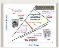
The figure shows an example of how the defect structure in laser powder bed fusion machines varies in a systematic but highly non-linear manner across power-speed space. In one corner, lack of overlap of melt pools induces lack-of-fusion...
