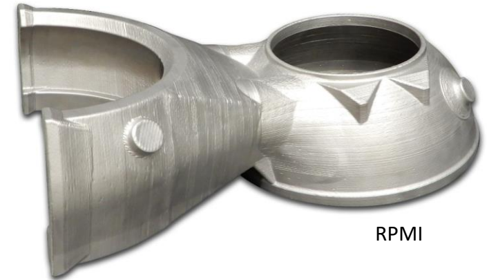
Multi-material combination with L-PBF and DED (RAMPT Project)
