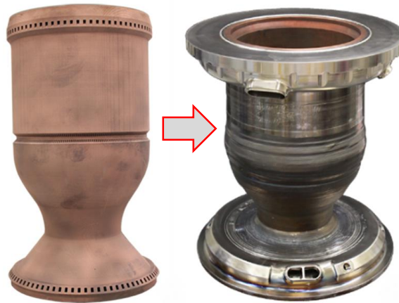
EB-DED Inco 625 Jacket on L-PBF GRCop-84 Liner
