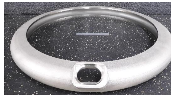
JBK-75, IN625, NASA HR-1 Manifolds
