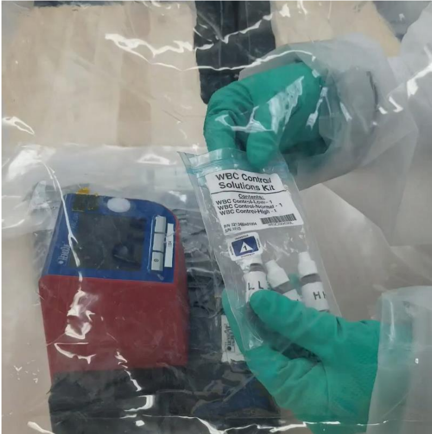
[Preparing a sample for ground testing with HemoCue® Analyzer]
