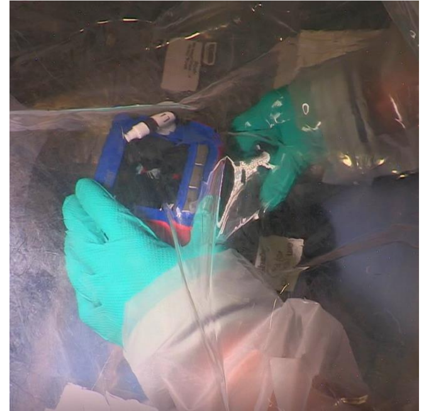
[HemoCue® Analyzer measuring a sample in the ISS Portable Glove Bag (IPGB) on-orbit]
