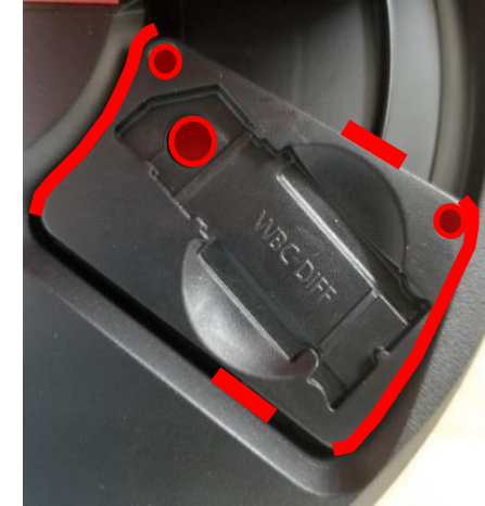
[Empty cuvette tray magnetically attached to the track of the analyzer base]
