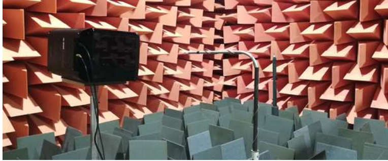
Figure 4: Photo of the free-field measurement setup. On the left is the Mackie HR824MK2 speaker, in the middle is the reference microphone used to validate the speaker output, and on the right is the microphone used as the free-field comparison for all results in the anechoic chamber.
