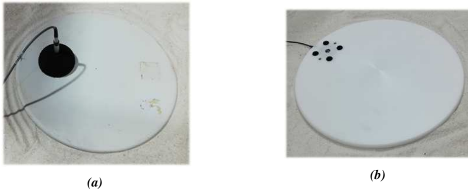
Figure 1: Microphone configurations showing (a) B&K 4964 microphone inverted over a ground board and (b) GRAS 67AX microphone embedded within a ground board and without the wind screen.
