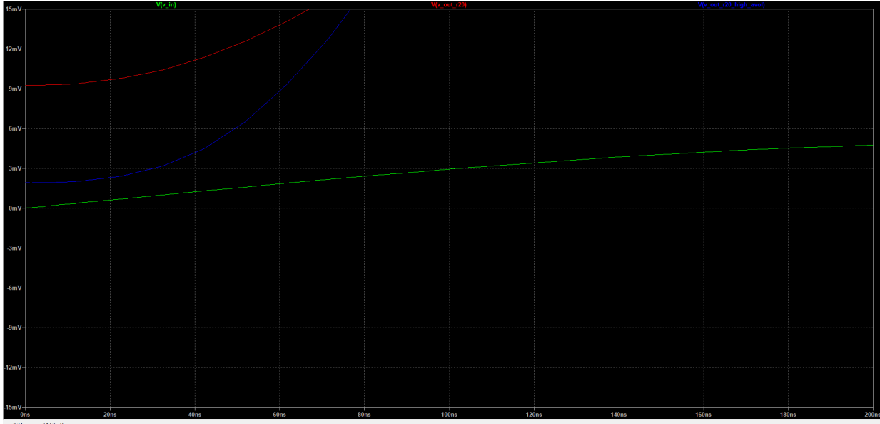
Figure 37.—Magnified detail of Figure 36 SPICE simulation waveforms comparing the DC offset of the single-stage (red) and two-stage (blue) output waves.
